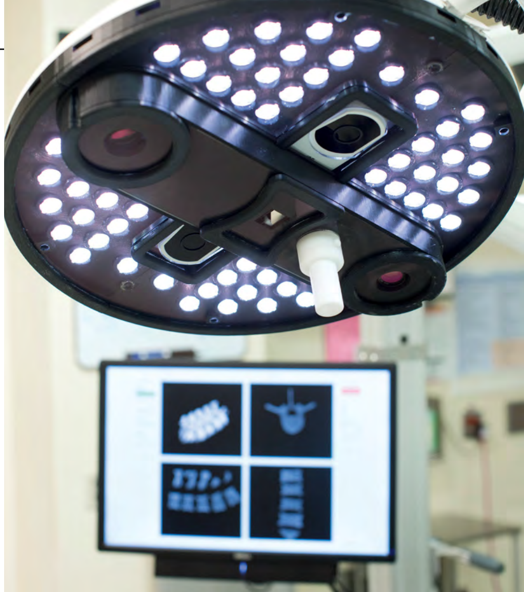
■ The light-based system that helps map the patient’s spine or brain to a high degree of accuracy.
