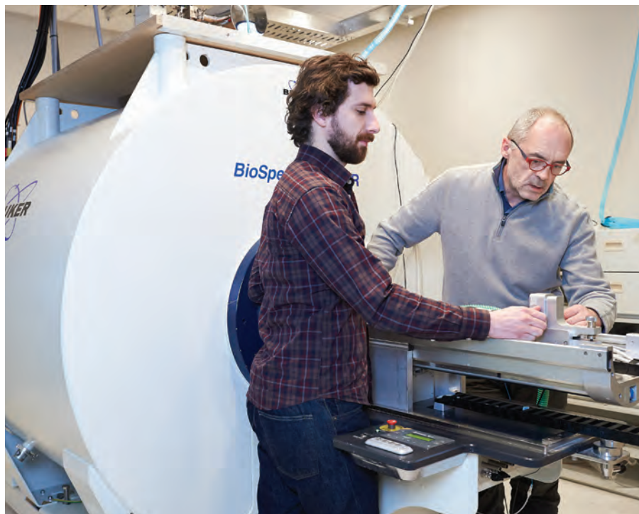
DR. GREG STANISZ (right) and his PhD student RAFAL JANIK work on a 7 Tesla magnetic resonance scanner. The researchers used this ultra-high-resolution imaging device to measure biochemical changes in the brains of mice fed bacterial supplements.
