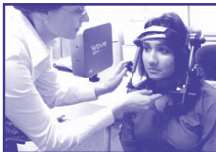
A 3D electromagnetic articulagraph (Wave Speech System, NDI, Canada) is used to measure the range of tongue and jaw movements in speech.
