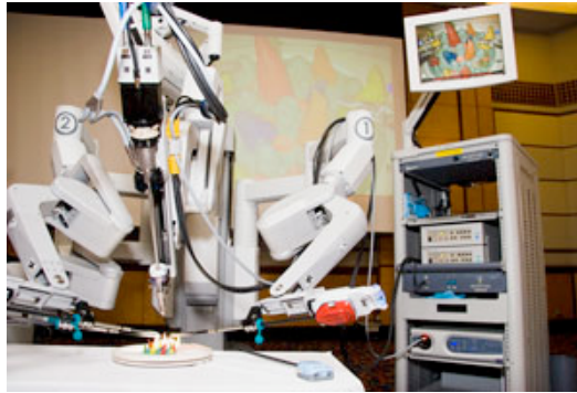
A full view of the da Vinci Robotic System
